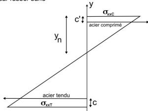
One can thus evaluate the position of the neutral axis of the beam  $y_n$  according to the position of steels. For that, should be solved the following equation:
