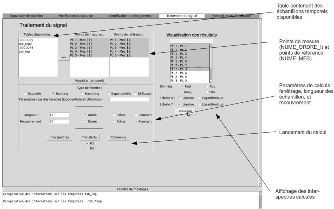
Figure 7-1: Mitre "Treatment of the signal" of the IHM CALC\_ESSAI
