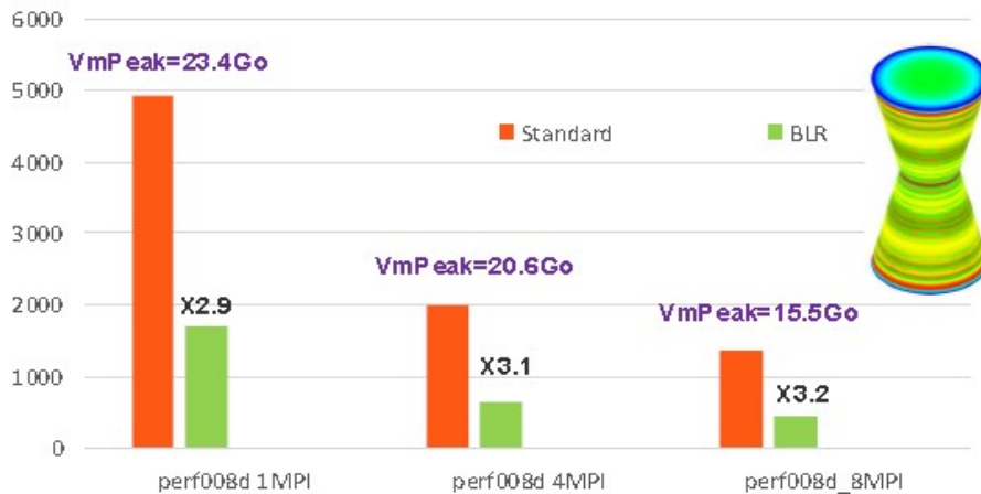
Figure 7.2-2: Example of profits gotten by compressions low-rank on the case benchmark perf008d (parameters by default, management memory in OOC, N=2M , NNZ=80M , Facto\_METIS4=7495M , conditionnement=10^7 ). One traces, according to the number of activated processes MPI, the times elapsed spent by all the stage of resolution of system linear in Code_Aster v13.1, his peak RAM report, as well as the factor of acceleration gotten by BLR.
