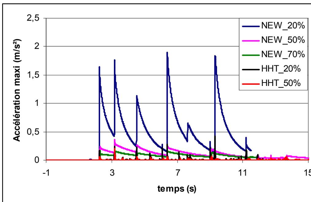
On the following figure, one can judge influence of a parameter of the discretization: the step of time, in term of control of maximum acceleration. The value of  $10^{-3}$  S for the step of time is not quite selected and it is then preferable to divide the step of time by two. To analyze this behavior, it is essential to conduct a parametric study on the step of time.
