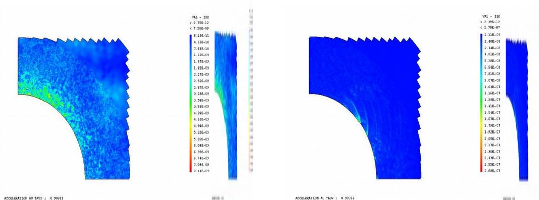
On the figure of left, one is in a weak phase of acceleration (non-linearity related to the rate of déconfinement is still low). The pace of the field of acceleration is rather random: one cannot perceive "reason" betraying a real dynamic phenomenon.
