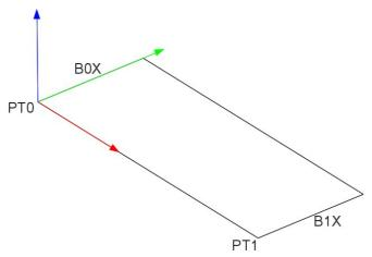
Pave:  $5\text{m} \times 3\text{m}$ , of thickness  $0.25\,m$ , on simple bearings in B0X and B1X. Higher three-dimensions function of reinforcements:  $8\,\phi\,12 = 9.0478\,cm^2$ , coating of  $2.5\,cm$ . Lower three-dimensions function of reinforcements:  $8\,\phi\,25 = 39.27\,cm^2$ , coating of  $2.5\,cm$ .
