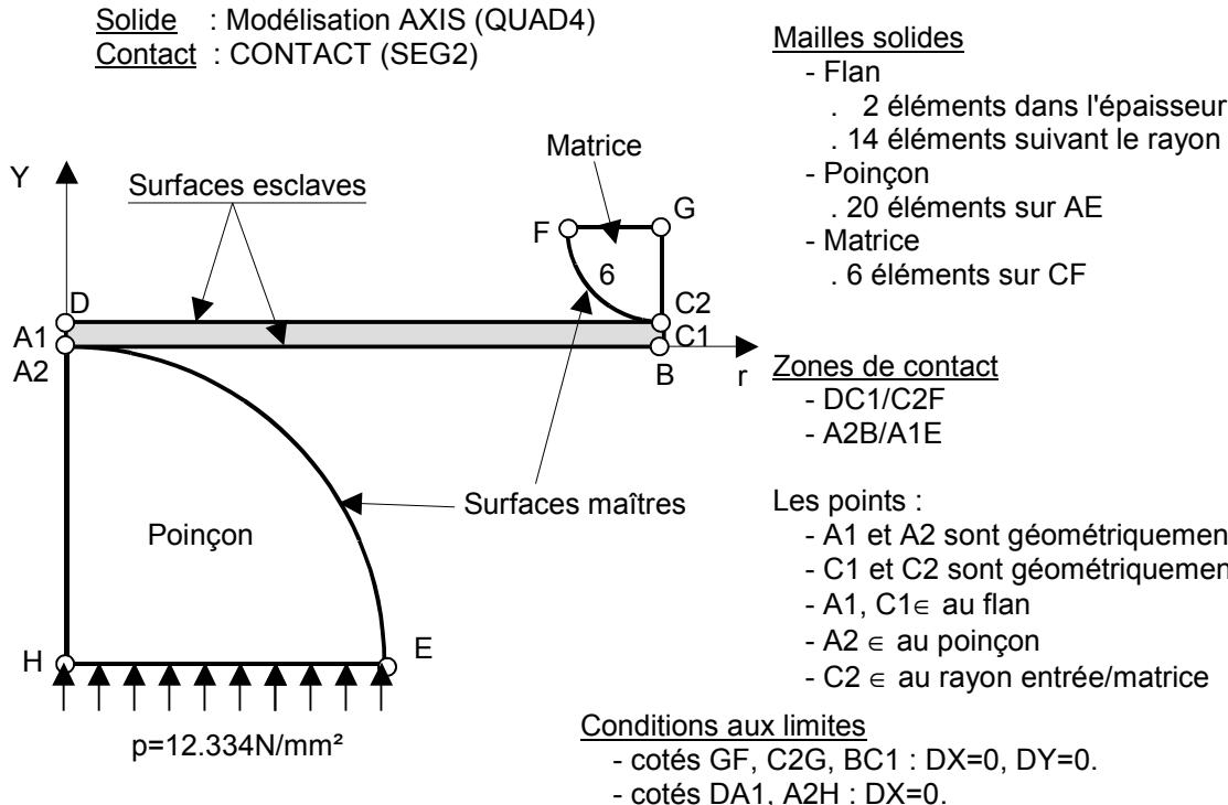
to avoid motions of rigid bodies, one imposes that displacements  $DY$  of the points  $A1$  (belonging to blank) and  $A2$  (belonging to punch) are identical.
