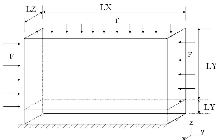
the structure is a healthy parallelepiped, into which a crack will be introduced directly into card-indexing it of command using operator DEFI\_FISS\_XFEM [U4.82.08]. The crack is present at a distance  $LY = 40\text{mm}$  from higher edge of the plate.
