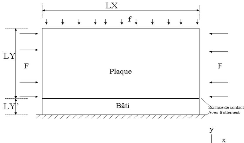
the structure is a rectangle made up of two of the same plates material, separated by an interface.
