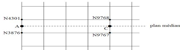
Figure 4.2-a : 4.2-a Conditions of Dirichlet around the median plane
