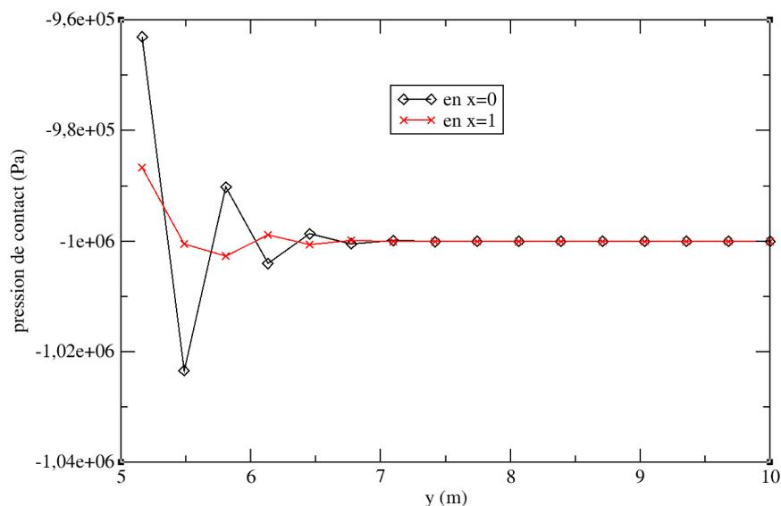
Figure 8.2 -8.1.1-a : Evolution of the contact pressure along the crack
