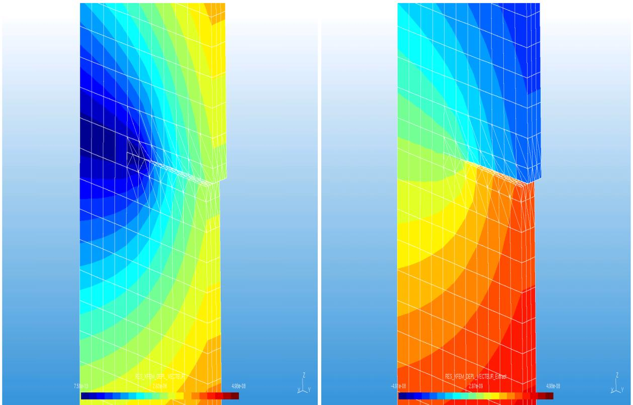
Appear 13.3.4-a : visualization of displacement (magnitude on the left, component DX on the right)
