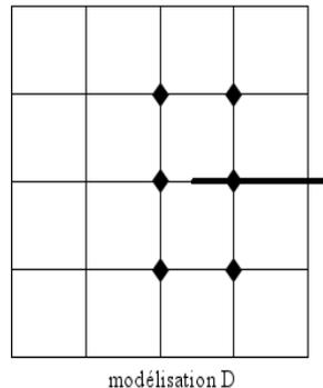
Figure 4.5 -5-a : Enrichment in a zone close to the crack tip
