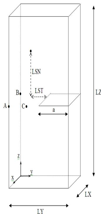
Appear 1.1-a : Geometry of the fissured plate
