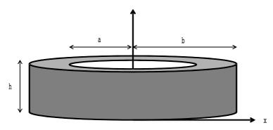
the cylinder has an interior radius  $a=10\,m$ , an external radius  $b=20\,m$ , a height of  $h=0.02\,\mathrm{m}$ the circumferential reinforcement, positioned on surface external of the cylinder, has a section per unit of length of  $s=0.1 \, m^2/ml$ . The principal direction of reinforcements is vertical.
