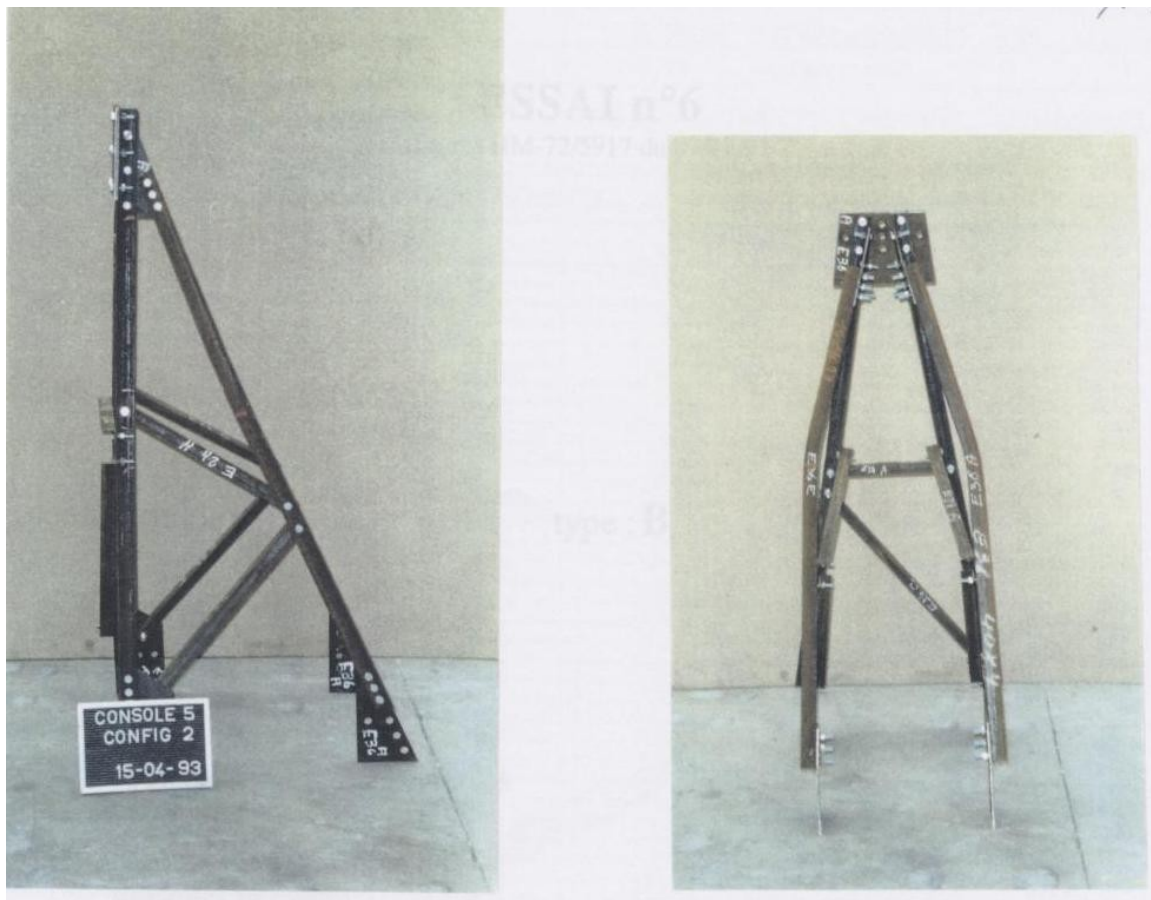
Appears 4.4.4-b : Mode of failure observed during the tests in configuration C2
