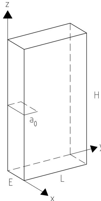
Appears 1.1-a: geometry of the fissured plate
