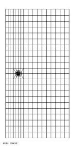
This modelization makes it possible to test the computation of Kl using POST\_K1\_K2\_K3 (method of extrapolation of displacements on the lips of crack) into axisymmetric.
