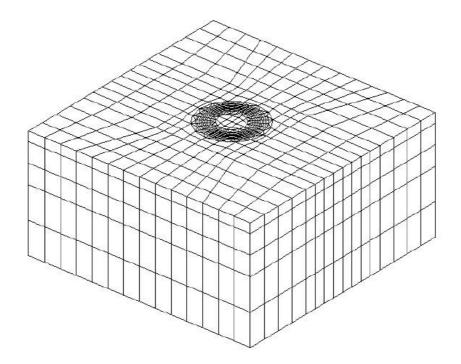
the interest of this modelization is to represent the entirety of the crack tip which is a closed curve, without benefitting from symmetries of the problem.
