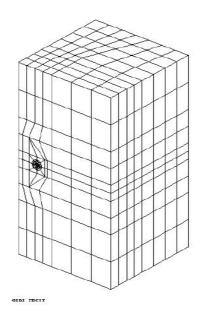
This modelization makes it possible to test the computation of KI using POST\_K1\_K2\_K3 (method of extrapolation of displacements on the lips of crack). Parameter ABSC\_CURV\_MAXI of the operator is calculated in POST\_K1\_K2\_K3 so as to retain 5 nodes on the segment of extrapolation ( dmax = 0.35).
