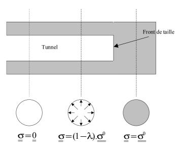
The solution of the problem is thus similar to that of the infinitely thick tube charged by an internal pressure with intensity  $(1-\lambda)\sigma_0$  and an external pressure with intensity  $\sigma_0$  (see [bib3] for the detail of computations).
