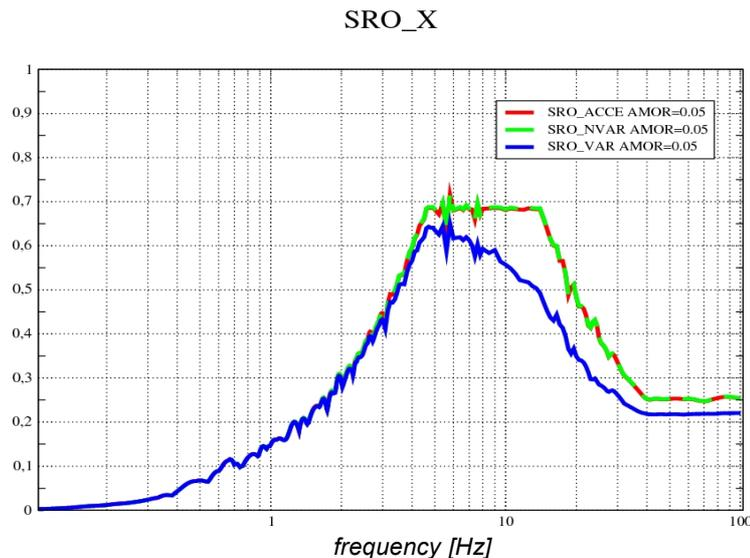
Note: For the case test, time step of the Euro accelerogram was multiplied by 2 (0.013672s instead of 0.006836s) in order to accelerate computations. Also, the SRO calculated in `sdls118b`, go from 0 to 50Hz and not from 0 to 100Hz as on the figure above.
