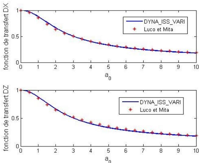
For the case  $\alpha=0.0$ , one tests the response after projection on physical coordinates. The rigid and massless foundation being, all the nodes undergo the same displacement which is equal to 1.0 in direction  $x$  for an excitation in direction  $x$ .
