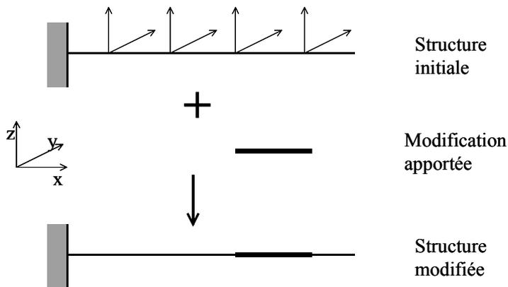
On the diagram above, the points of measurement on the structure initial are materialized by deflections, of which the point indicates the significant direction of the sensor. These points of measurement are localised with the X-coordinates  $0.2m$ ,  $0.4m$ ,  $0.6m$  and  $0.8m$  according to the directions  $y$  and  $z$ . Measured information is available only in these points of measurement.
