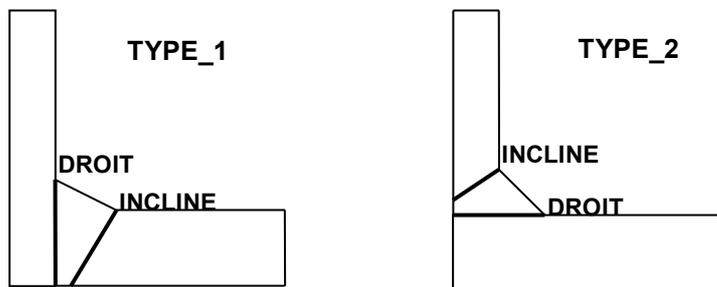
Appears 4.7.13-a: Definition of the position of a crack according to the type of the weld
