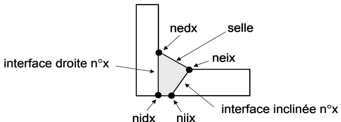
**Appear 5-b: Names of the nodes groups to the azimuth  $n^\circ x$  of the operational bypass**
