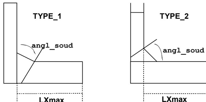
Figure 4.4.8-a: Definition of the position of the weld
