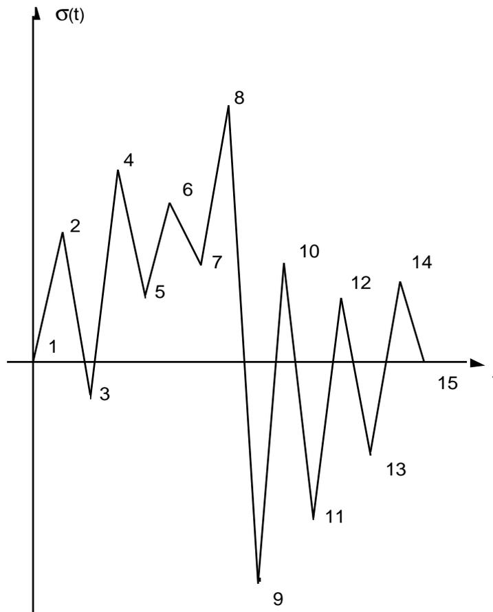
The load history being composed of 15 points, the method "naturalness" determines 7 elementary cycles:
