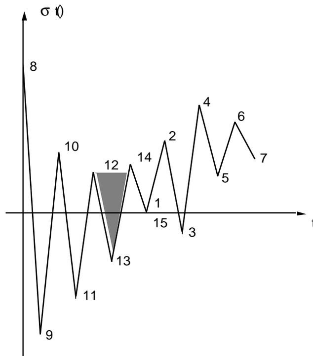
The second stage consists in extracting the elementary cycles. The first extracted cycle is the cycle defined by items 12 and 13 since  $|\sigma(12) - \sigma(13)|$  is lower than  $|\sigma(14) - \sigma(13)|$  and  $|\sigma(12) - \sigma(13)|$  is lower than  $|\sigma(12) - \sigma(11)|$ . Cycle
