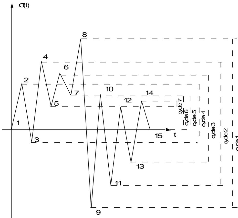
The first stage which consists in ordering the history of the loading, of smallest with the greatest value of the loading, conduit to following storage:
