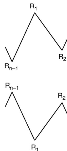
d) Raccordement transition ( $R_{n-1}, R_1$ ), on élimine  $R_n$
