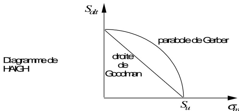
From a cycle  $(S_{alt}, \sigma_m)$  identified in the signal one calculates the value of the corrected alternate stress  $S'_{alt}$ .
