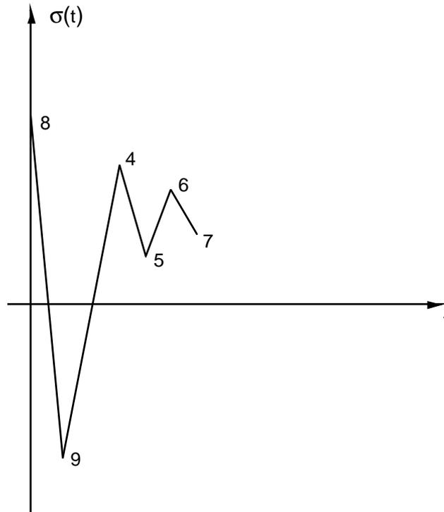
is noticed well that when one applies counting RAINFLOW to the whole made up of the two residues, one obtains in the end counting again the initial residue.
