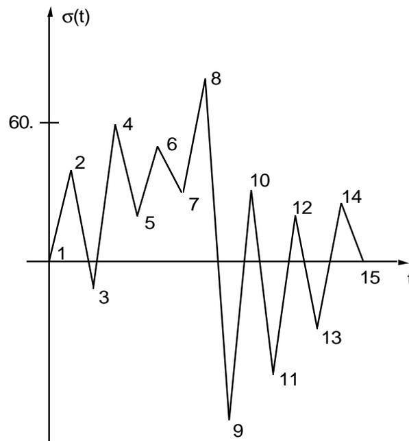
The method of RAINFLOW thus leads, on this example, (see [Annexe1], for detail of the stages of the algorithm) with the determination of 7 elementary cycles defined by the maximum value and the minimal value of the loading, for each cycle.
