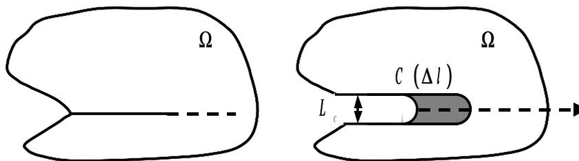
Appear 1.2-a - Representation of crack by a notch
