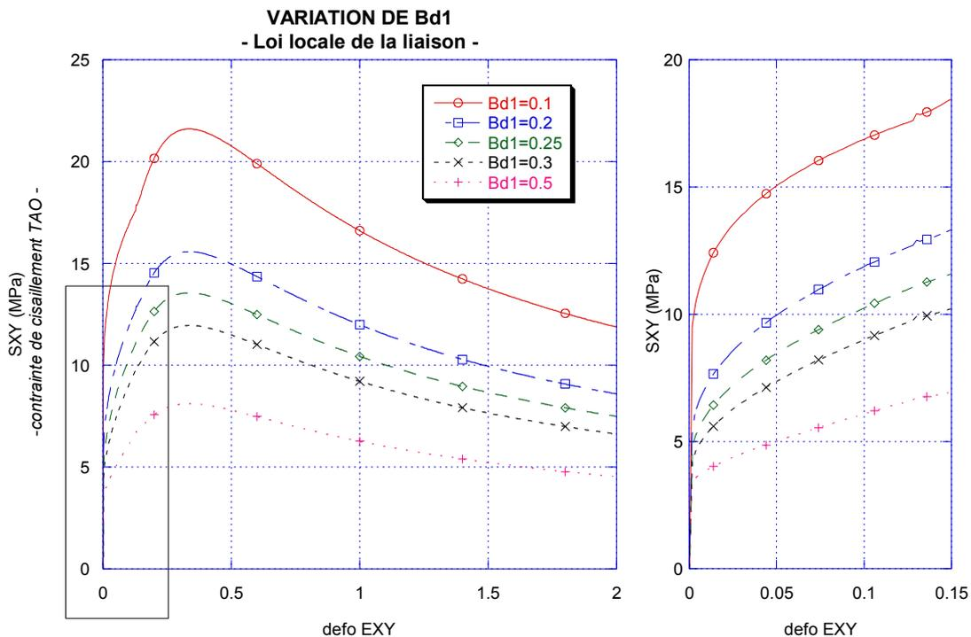
Appears 5.2.3-a: Comparison of  $B_{IDT}$  : Modification of the curvature
