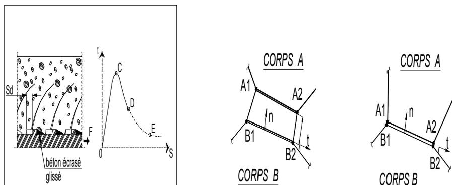
**Appear 2-a: real description of the phenomenon of connection and simplification finite elements: coordinated in the local coordinate system of the element of interface used as support of theoretical model**
