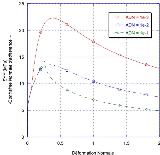
Appear 5.3.3-a: behavior of connection on the normal direction at the time of the opening of the interface (normal tension on connection).
