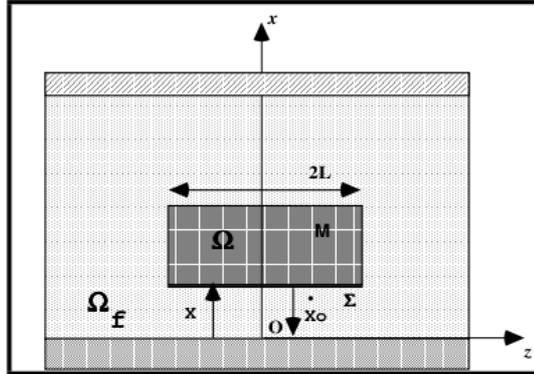
Appear 3-3-a3-a : Mass damped by a fluid blade
