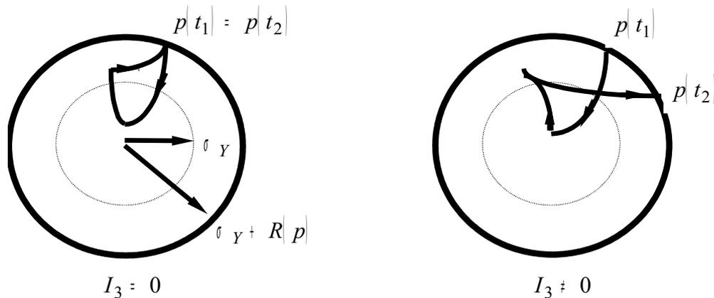
**Appeur 3.1-a : Loading path enters  $t_1$  and  $t_2$  in the plane deviatoric of the stresses**
