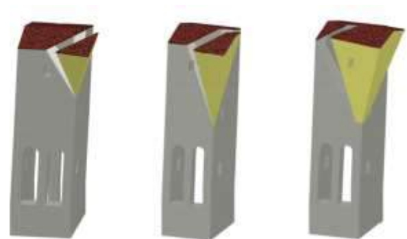
Analysed collapse mechanisms
