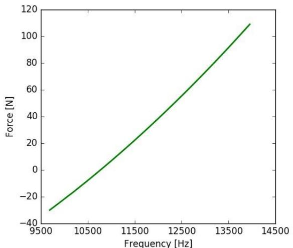
Figure 4: Simulated dependency of force and resonance frequency
