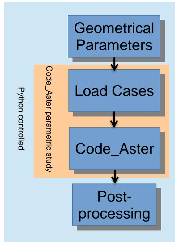
Figure 2: Structure of the simulation process
