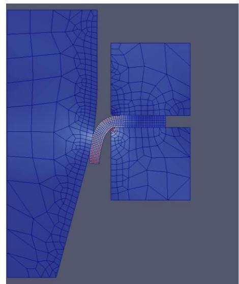
Figure 1: Axial symmetric simulation of the deep draw process
