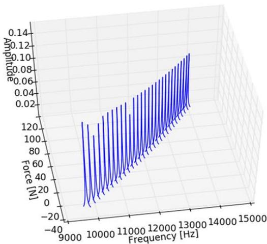
Figure 3: Harmonic response of different load cases
